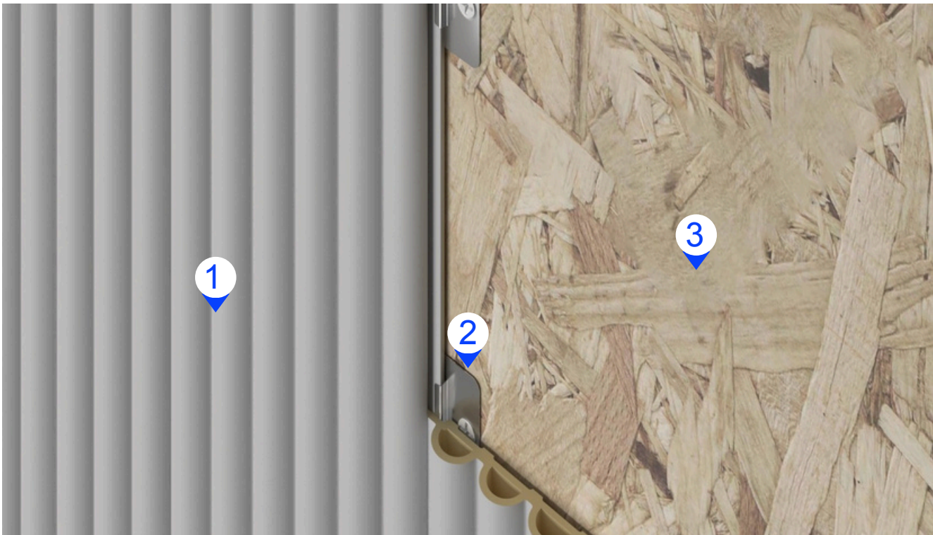
1. Apply structural adhesive on the back 2. Male and female slot splicing or metal clip splicing 3. Puttying and leveling
